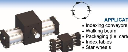
The Rotomation indexing actuator is a unique pneumatic device that reliably provides shaft rotation in precise steps in one direction without cumulative error. It shares a number of components with a normal rack and pinion rotary actuator.
